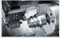
UNIVERSAL TURNING 6-sided complete machining of workpieces up to ø 366 × 708 mm and 120 mm Y-axis
