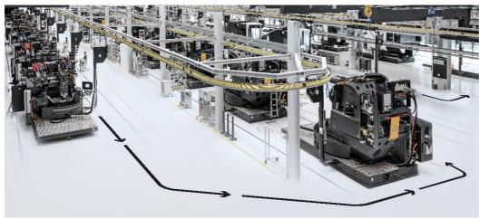
01 **Digital and automated:** the flow assembly with 34 AGVs in the new monoBLOCK Excellence Factory at DECKEL MAHO Pfronten increases productivity by 30%.
