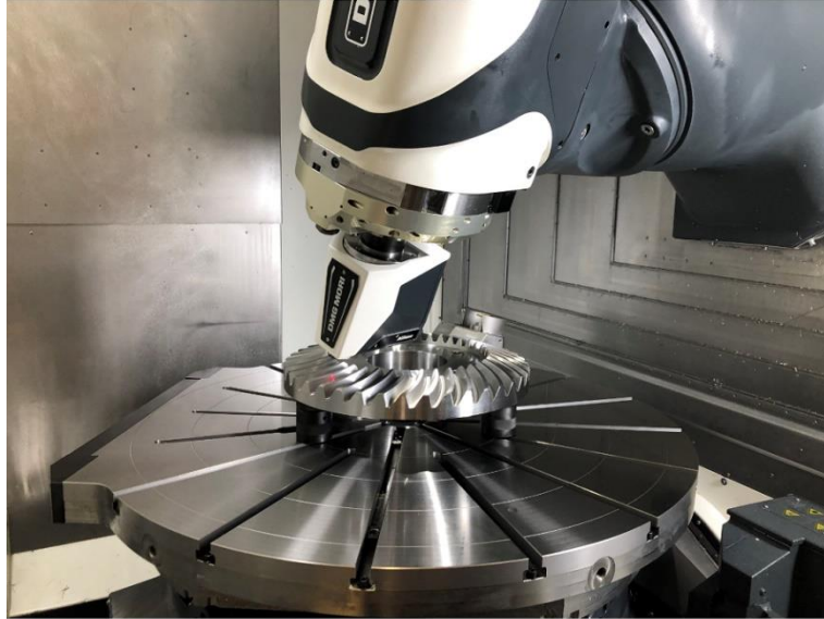
Image of the on-machine measuring system equipped with Nikon's non-contact laser scanner LC15Dx
