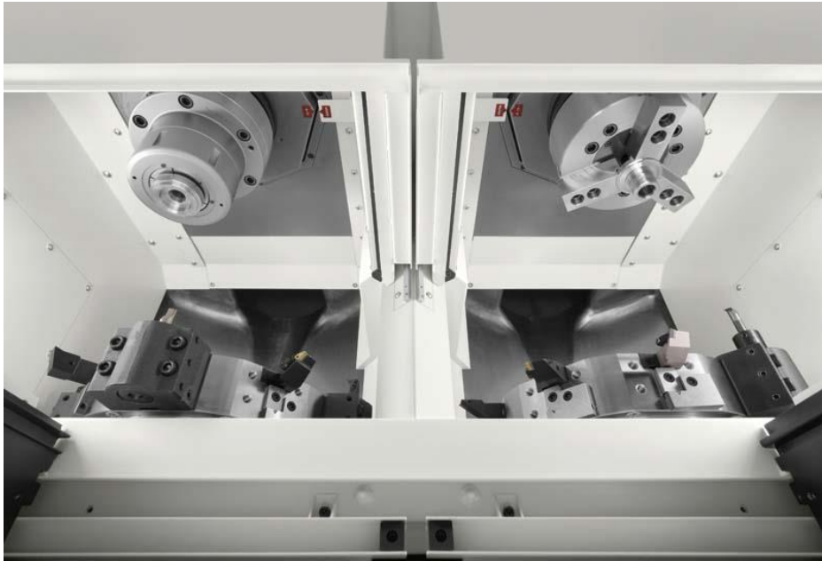
Photo 2: Built-in spindles and turrets
