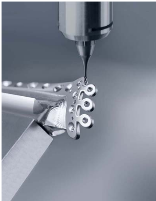
Photo 12. Machining of bone plate (HSC 20 linear )
