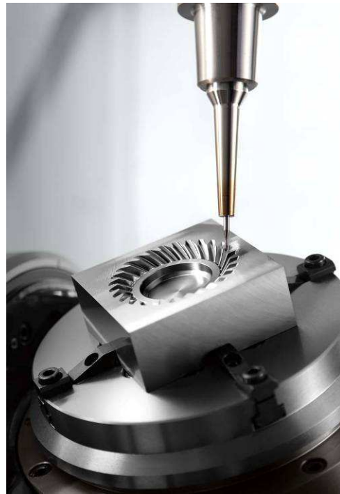
Figure 11. Bevel gear forging die (NVX5080 II/40 + 5AX-DDRT200)
