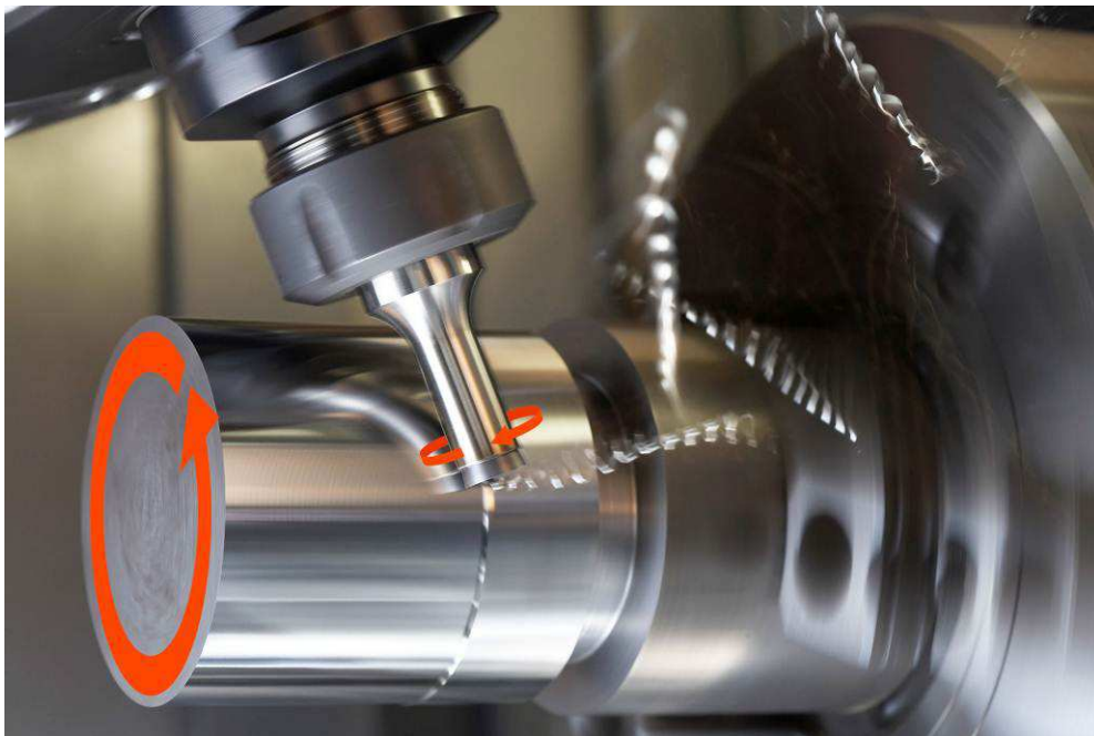
Figure 8. Machining with Spinning Tool
