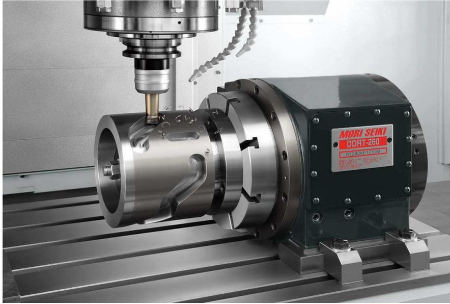
Fig.3 Machining with DDRT
