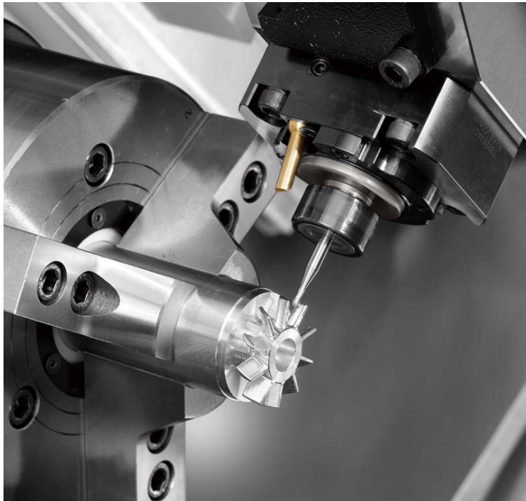
Photo 4: High-speed milling with a max. spindle speed of 10,000 min -1
