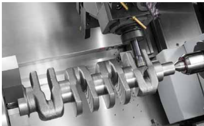
Figure 4. Machining example (crank shaft)
