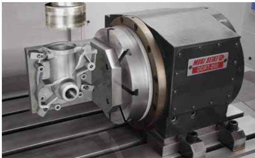
Fig 1. Machining Example (Water Pump)
