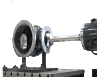
Large diameter boring using a boring spindle
