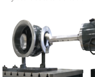
Large diameter boring using a boring spindle
