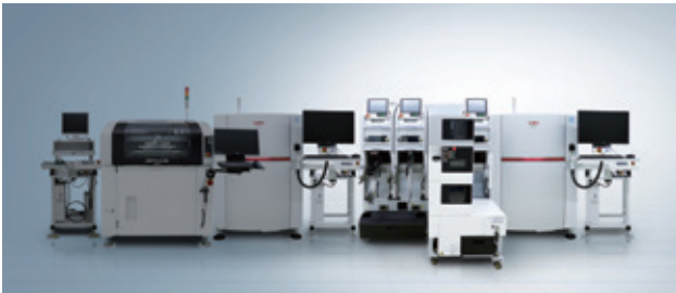
SMT line consisting of mounting and inspection machines
