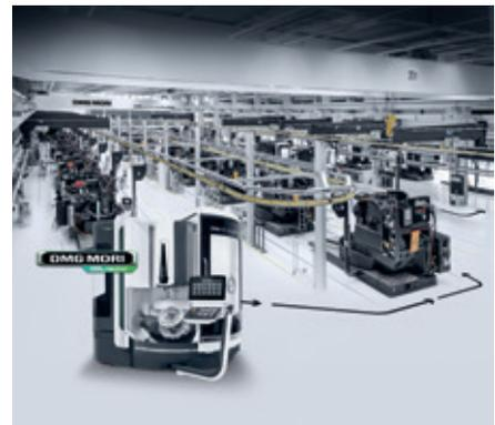
September 2020 marked the opening of the monoBLOCK Excellence Factory in Pfronten, Germany, DMG MORI's largest production site in Europe. The monoBLOCK Excellence Factory offers 4,000 m<sup>2</sup> of space for line production by AGVs (Automated Guided Vehicles), which improved productivity by 30%. As a result, the annual production capacity has expanded from 600 to 1,000 units.
