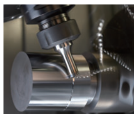
Cutting with the Spinning Tool
