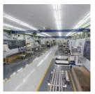
Ball Screw Plant: male thread-grinding line
