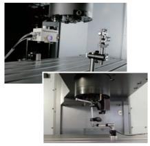
Laser measurement (upper), and DBB measurement for roundness
