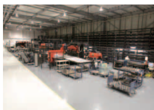
Sheet Metal Plant: automatic sheet metal manufacturing system (left) and YAG welding robot (right)
