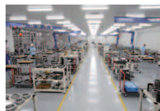
Spindle Plant: the Clean Room, where temperature, humidity and cleanliness are strictly controlled.
