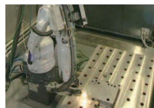
Sheet Metal Plant: automatic sheet metal manufacturing system (left) and YAG welding robot (right)
