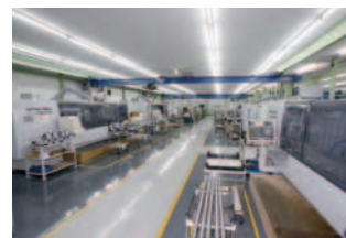
Ball Screw Plant: male thread-grinding line
