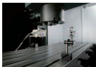
Inspection before shipment using laser measurement
