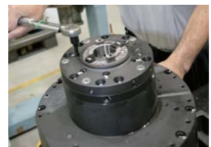
Assembly of spindle units using the cell production system
