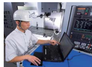
Inspection of positioning accuracy and repeatability using a laser measuring device
