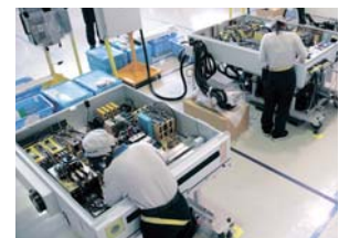
Assembly line for electrical cabinets
