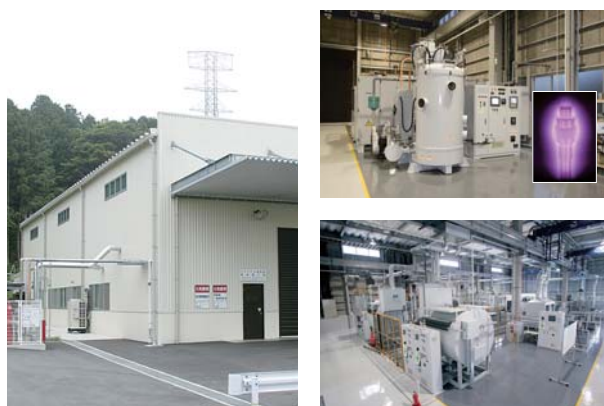
Left: Heat Treatment Plant Top right: Ion-nitriding system and inside view Bottom right: Carburizing and quenching furnace
